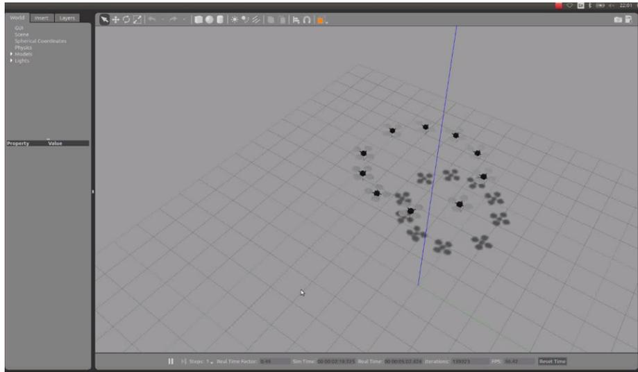
Figure 7: Quadrotors following the limit cycle of the nonlinear parabolic potential swarm in Gazebo. The agents are controlled by ROS, which is feeds velocity and position data between Gazebo and Mathematica. Note the similarity to the limit behavior pictured in Figure 1.
